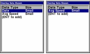
Overlay Data Shown, with Date option selected (left). Overlay Data Shown menu with Date Removed from the list (right).
